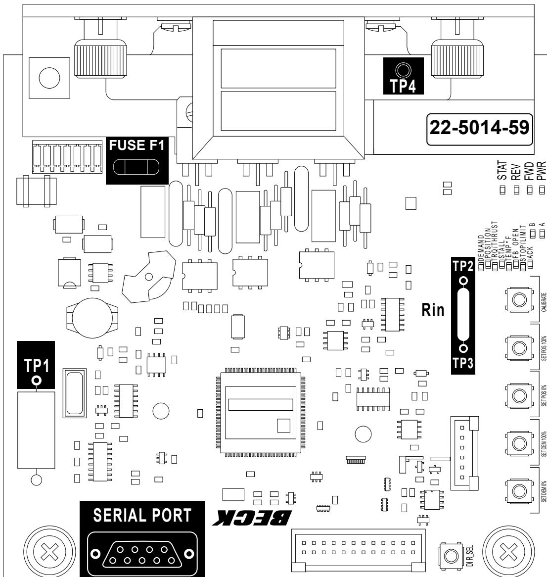
The DCM-3 provides voltage test points allowing the verification of the demand signal and position signal at the DCM-3 board.
