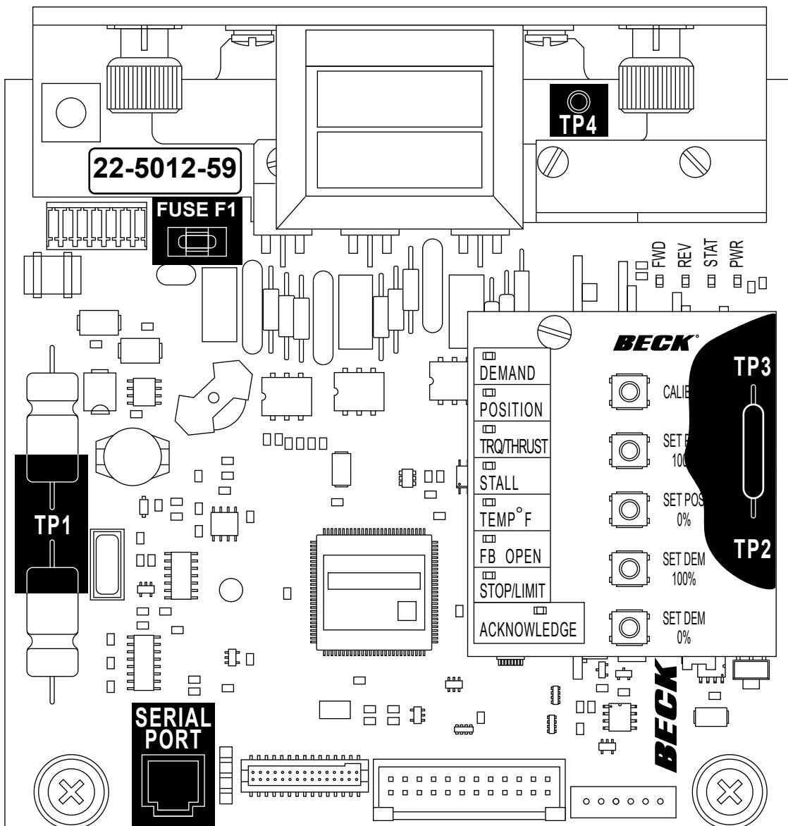
The DCM-2 provides voltage test points allowing the verification of the demand signal and position signal at the DCM-2 board.
