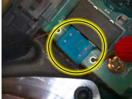
“BLADE-TYPE” FUSE (TOP VIEW)
