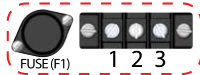
As Supplied With Optional Transformer for 208, 240, 380, 416, 480, & 575 Volts
