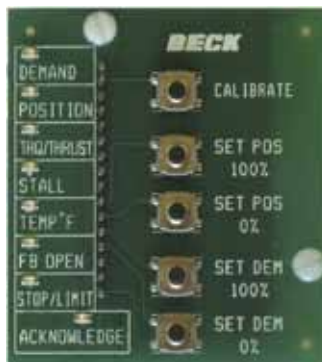
DCM-2 Pushbutton Panel
